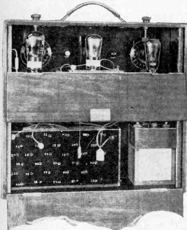
Interior of the "Advance" portable, showing tuning dials and readily accessible grid battery.
