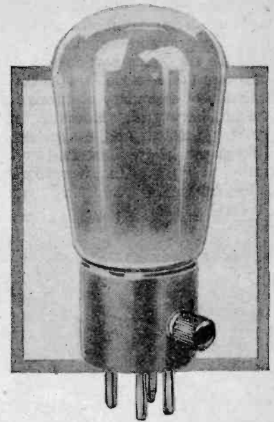
The Mullard pentode power output valve. The four-volt type illustrated above (P.M.24) has a filament consumption of 0.15 amp. The maximum anode potential is 150 volts at which the makers claim that a total grid swing of about 21 volts ( \pm 10.5 ) can be accommodated and that the mutual conductance is 2.3 mA per volt.
