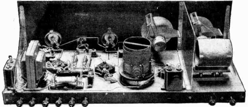
The "Standard Four," as constructed by a reader. Faults were located in the base of the aerial-grid coil, which is seen at the extreme right-hand side of the photograph.
